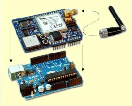
The *GSM/GPRS/GPS-Shield* is plugged as "primary" shield on top of the *Arduino* board, ensuring that the antenna of the integrated GPS receiver has "free view". The communication between the two boards is achieved via the serial interface (GSM/GPRS) and SPI (GPS).
